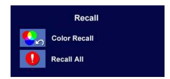
Press the  $\blacktriangleleft$  or  $\blacktriangleright$  keys to select **Color Recall**. Press the **Enter** key to recall color settings, or press the **Exit** key to return to previous menu.
